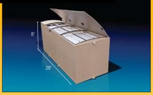
A full-sized 42' long AdvanTex-MAX unit can be configured as a 15,000 gpd treatment system when receiving primary treated effluent from septic tank(s) or an effluent sewer. Alternatively, the same unit can be configured as a 5000 gpd system when receiving raw sewage. Smaller (shorter) units are available for smaller flows and mobile treatment systems.
